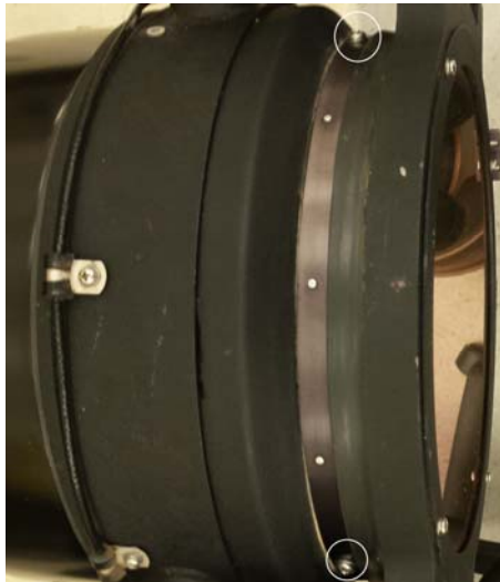
Figure 48 IFCO Hood Showing the Fasteners at 2 and 10 o'clock positions
